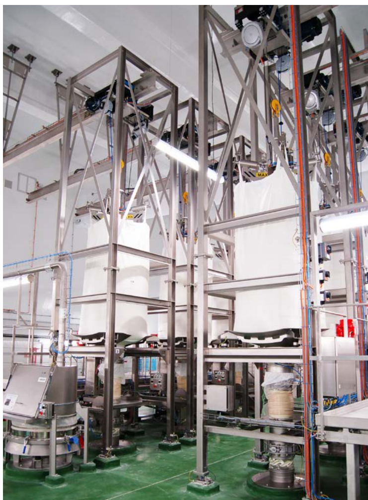
Lean Gravity Mixing met high care big bag handling
